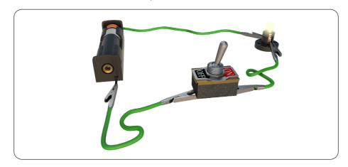
When electricity cannot flow through all the components of a circuit, it is called an incomplete circuit. Loose wires, damaged components and flat cells or batteries can all stop the flow of electricity around a circuit.
